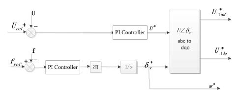
Figure 3. V/f controller structure
