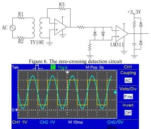
Figure 7. The measured waveform of zero-crossing detection circuit
