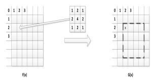
Figure1. Gaussian pyramid filter 3x3 kernel
