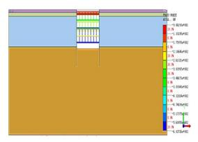
Figure 7. The original scheme supporting axial force cloud
