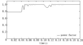
Figure 15. Power factor variation before and after compensation
