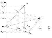
Figure 8 .The voltage and current vector in the  $\alpha\beta0$  coordinate system Suppose three-phase voltage and current instantaneous values are respectively ua, ub, uc, ia, ib, ic. ua, u $\beta$ ,
