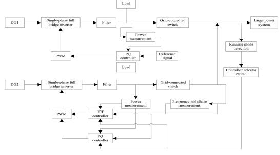
Figure 1. The control diagram of modules in microgrid system
