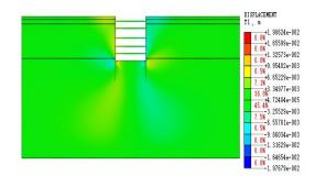
Figure 3. The changed plan of underground diaphragm wall lateral contours
