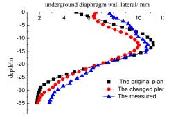
Figure 4. The lateral curve of underground diaphragm wall
