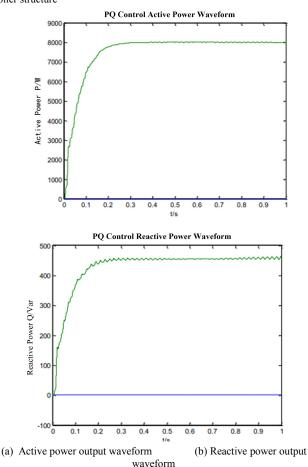
Figure 5. PQ control active power and reactive power output waveform
