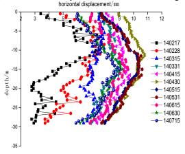
Figure 5. The measured later curve of underground diaphragm wall
