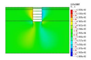
Figure 2. The original plan of underground diaphragm wall lateral contours
