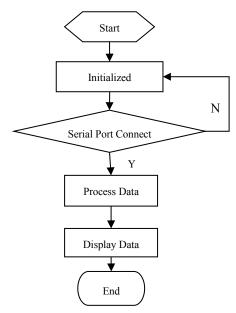
Figure 8.the host pc design flowchart
