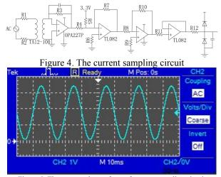
Figure 5. The measured waveform of current sampling circuit
