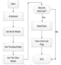
Figure 7.the flowchart of receive packet
